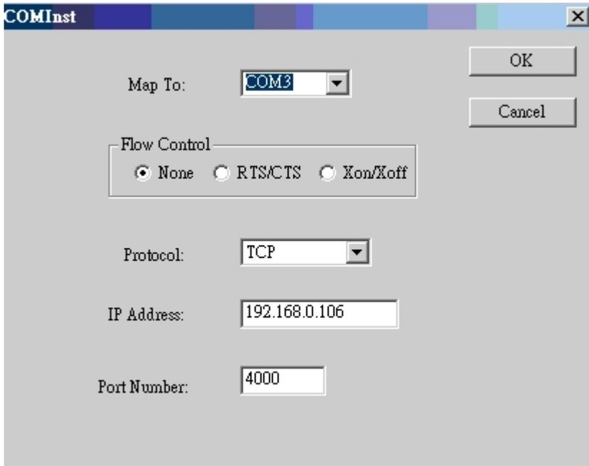
**Note1.** If any settings are changed in this part of the Virtual COM setup, it will only affect the settings in the operating system Device Manager. It will not change the settings in the TRP-C32.
