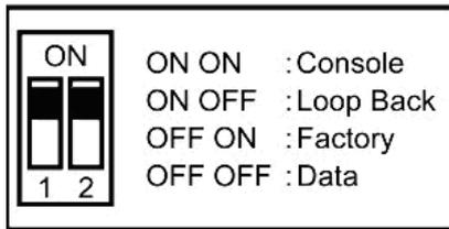
When all these switches are moved into the ON position, the TRP-C32 enters Console Mode, allowing configuration of the TRP-C32 from a PC running a terminal program such as Hyper-terminal. When the TRP-C32 enters Console Mode, the Console Mode screen will appear in the Hyper-terminal program window. The serial port settings must be 8-N-1 at 9600 baud.
