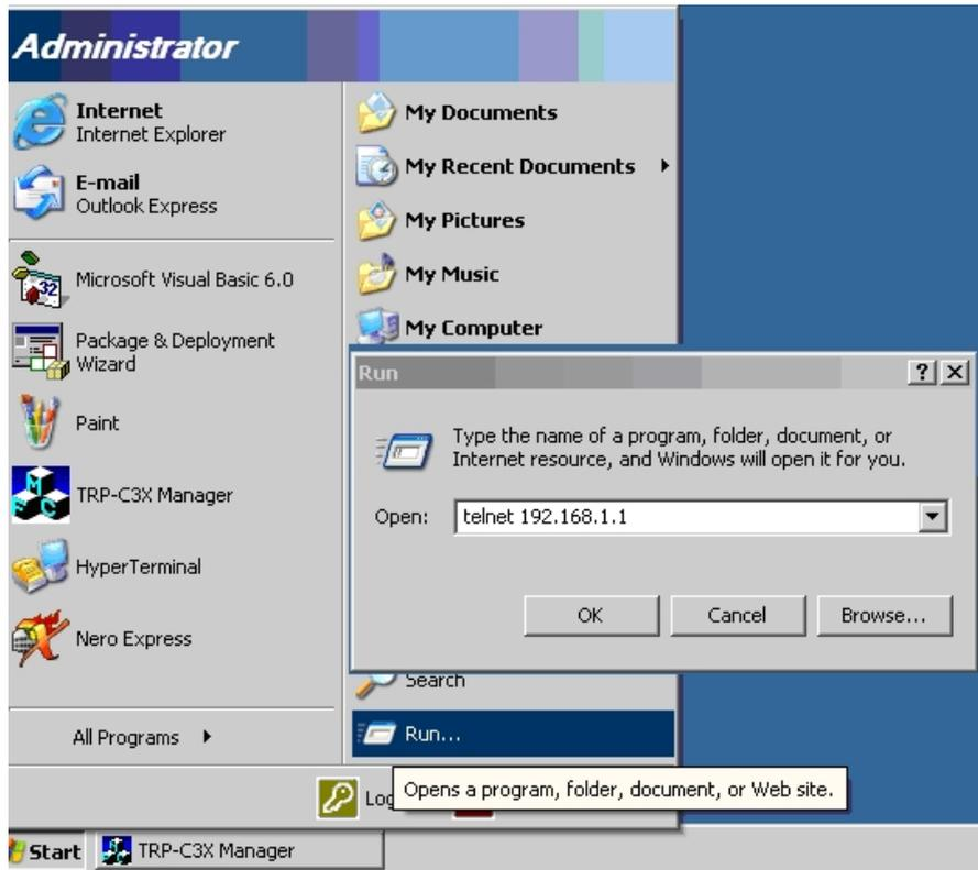
**STEP2.** Click the “OK” TRP-C32 firmware setting will show as following screen. You can set the TRP-C32 by Telnet mode.
